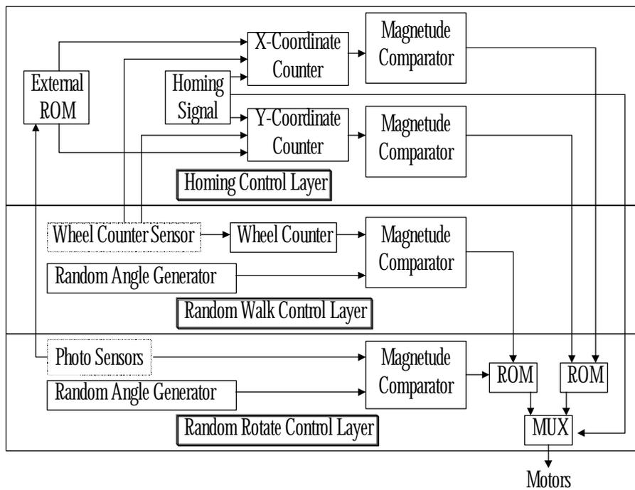
Figure 2. Logical design of the behavioral control chip
