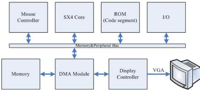
Figure 1. System overview of the proposed processor.
