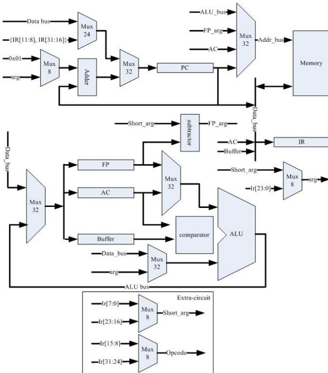
Figure 2. The data path of the proposed processor.
