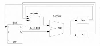
Figure 3. Hardware Organization of processing element
