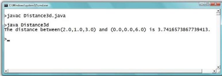
**Figure 55: The output of the Distance3d program**
