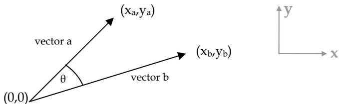
Figure 130: Two vectors in the Cartesian coordinate
