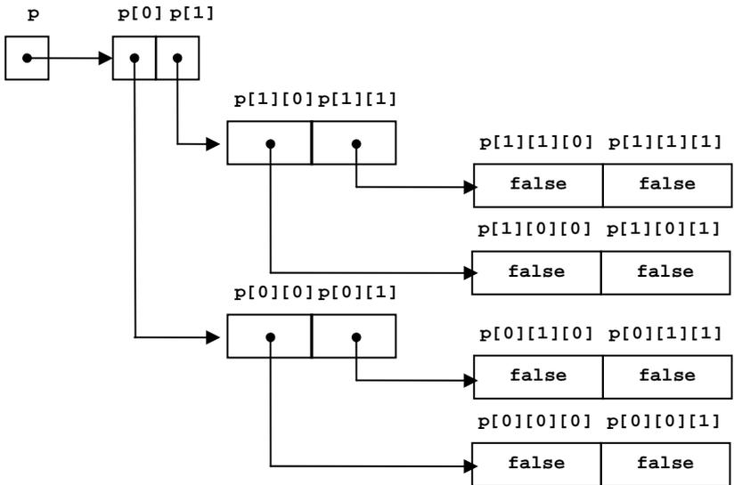
Figure 160: A three dimensional array of boolean
