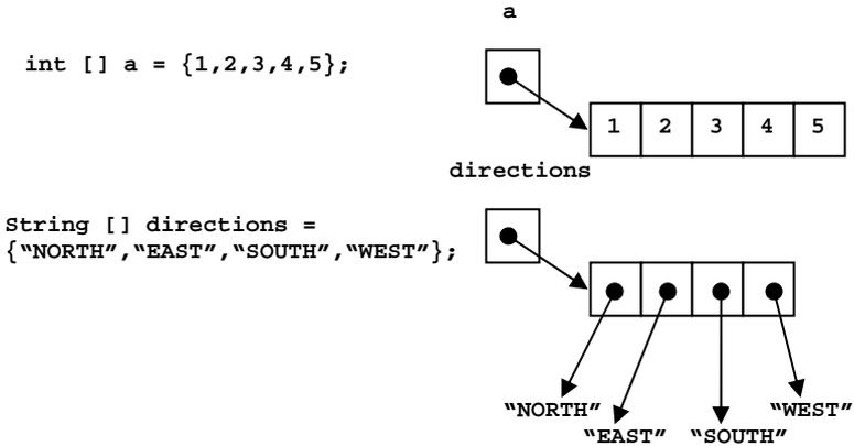
Figure 148: Illustration of some usage of initializer lists
