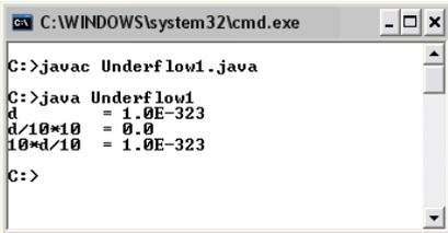
Figure 62: A demonstration of cases when underflow occurs
