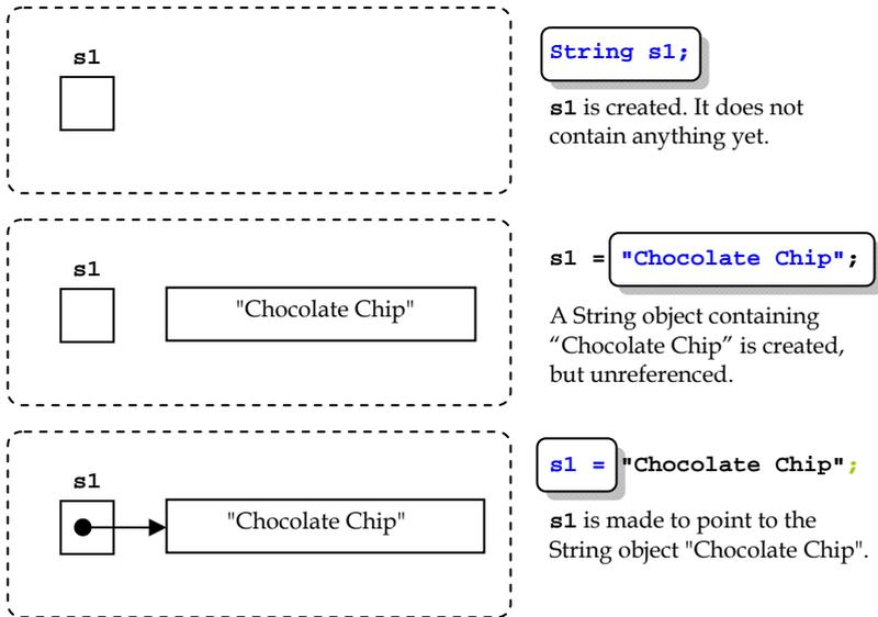
Figure 68: Declaration and assignment of a String object
