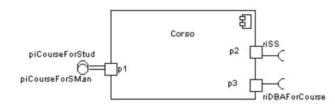
If there are multiple interfaces associated with a port, these interfaces may be listed with the interface icon, separated by a commas
