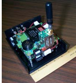
(a) The SCADDS PC/104 node
