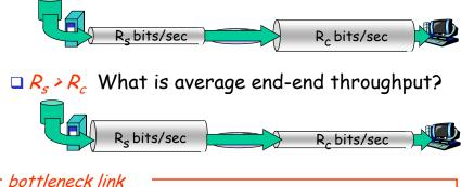
link on end-end path that constrains end-end throughput
