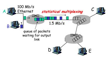
Sequence of A & B packets does not have fixed pattern, bandwidth shared on demand → statistical multiplexing.
