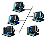
shared wire (e.g., cabled Ethernet)
