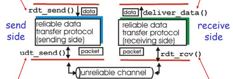
**udt\_send():** called by rdt, to transfer packet over unreliable channel to receiver
