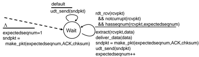
ACK-only: always send ACK for correctly-received pkt with highest *in-order* seq #
