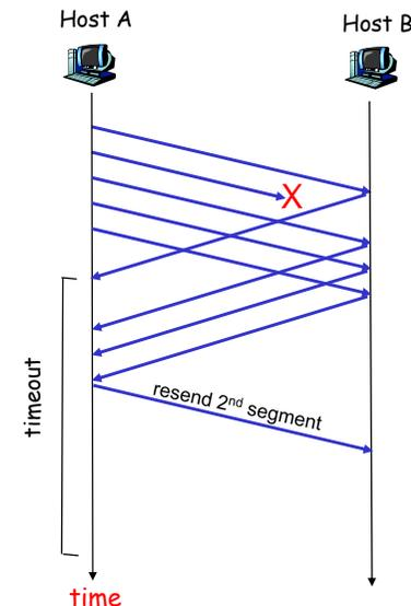
Figure 3.37 Resending a segment after triple duplicate ACK
