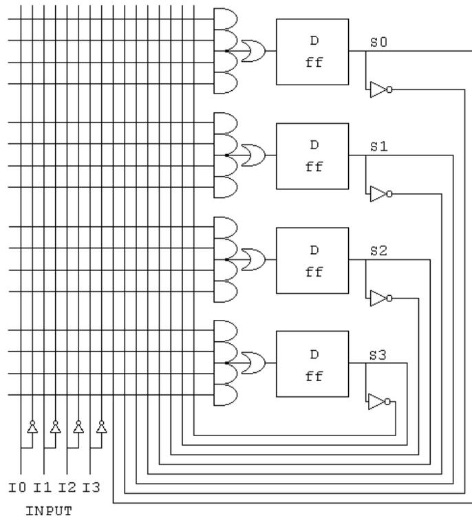
Figure 2. GAL structure used in the experiment
