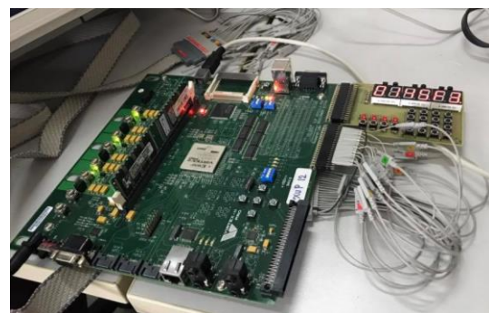
Fig. 4. Implementation of TX on XUP Vertex II Pro Board
