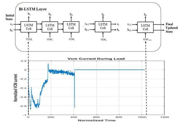
Fig. 8. LSTM Network Layer
