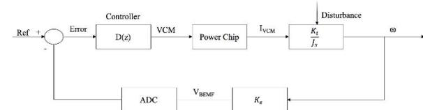
Fig. 2. Closed-loop control system of actuator arm.
