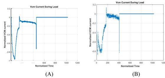
Fig. 5. (A) VCM current of good drive. (B) VCM current of bad drive.
