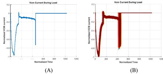
Fig. 3. (A) Single VCM current. (B) 1000x overlay of VCM current.
