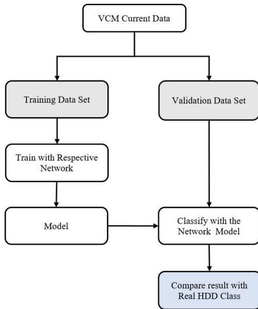
Fig. 7. Testing and validation work flow.
