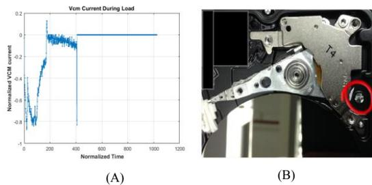
Fig. 4. (A) VCM current of missing latch drive. (B) Missing Latch position.
