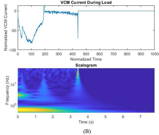
Fig. 11. Scalogram of a good drive (A) and a bad drive (B).
