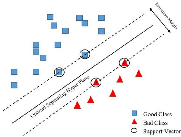
Fig. 12. Support Vector Machine for classification
