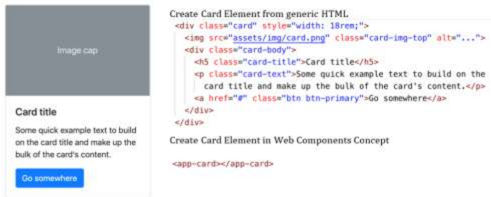
Figure 1: Compare to create card elements between generic HTML and Web Components concepts.
