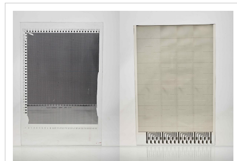
The prototypes [3] of the x-y mutual capacitance multi-touch screens (left) developed at CERN
