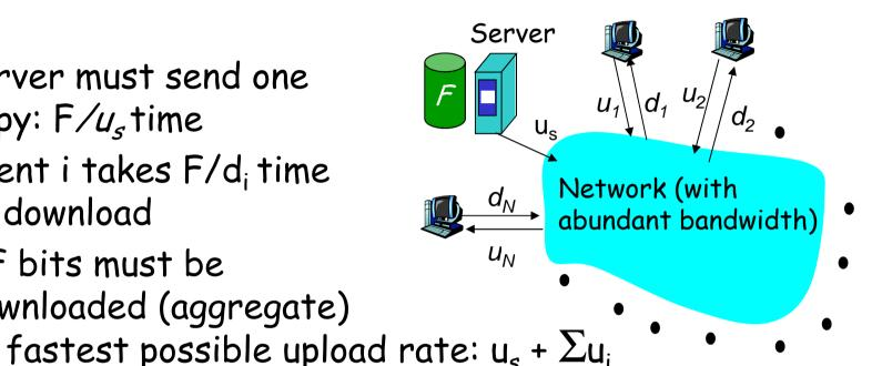
$$d_{P2P} = max \{ F/u_s, F/min(d_i), NF/(u_s + \Sigma u_i) \}$$
