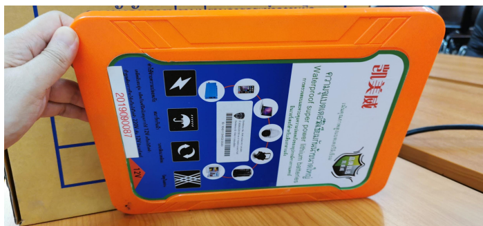
Figure B.1: One of the seized devices, disguised as a waterproof industrial battery pack. The label is a fabricated product sticker printed in Chinese; the actual contents are electronic circuits encapsulated in black epoxy resin.
