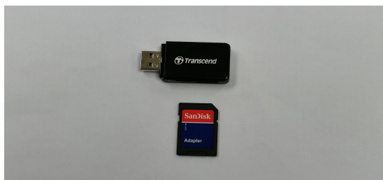
Figure B.4: The Transcend USB card reader and SanDisk microSD adapter used to connect the evidence card to the investigator's machine. The card was presented to the operating system in read-only mode throughout the imaging step.
