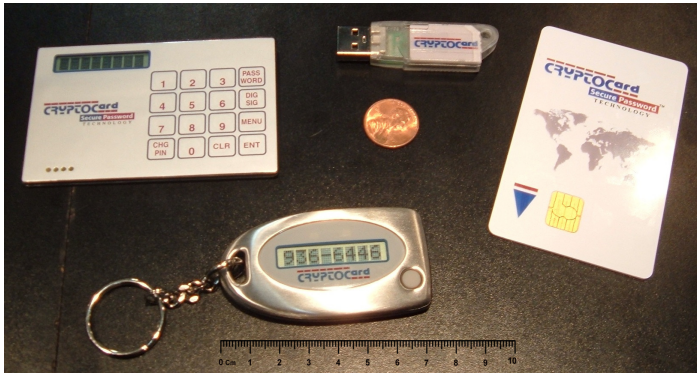
Figure 2.3: A CryptoCard one-time-password token. The device holds the shared secret and generates a fresh password for each login, so nothing reusable crosses the network.
