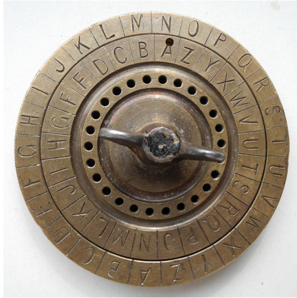
Figure 6.1: A cipher disc. Rotating the inner ring against the outer one fixes a substitution alphabet; the amount of rotation is the key.
