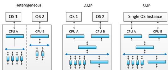
Fig. 2. Multicore processing system architectures
