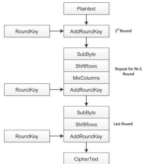
Fig. 1. AES Encryption flow
