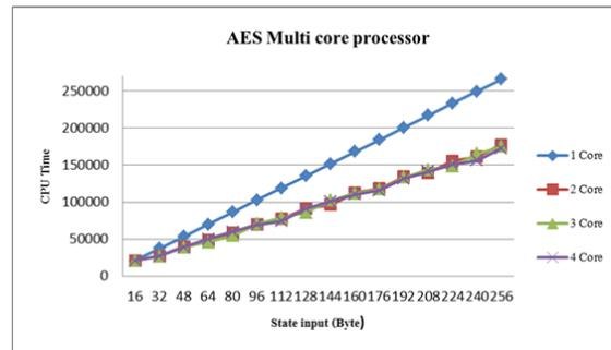
Fig. 5. The result of AES on single core and multi-core processor
