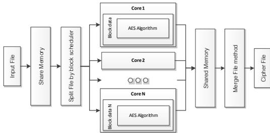
Fig. 3. AES algorithm on multicore processor
