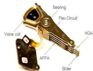
**Figure 1:** Diagram of a computer hard disk drive [13] **Figure 2:** Head Stack Assembly (HSA) [9]
