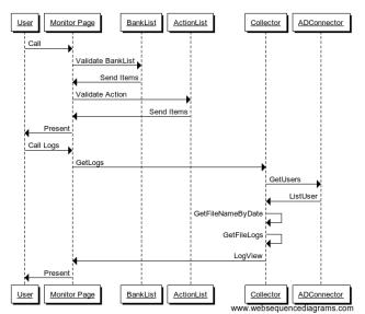
Fig. 1. Sequence diagram of Monitor Function
