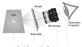
Fig. 3. Camera with x10 microscope.
