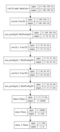
Fig. 6. Structure of model simple DCNNs.
