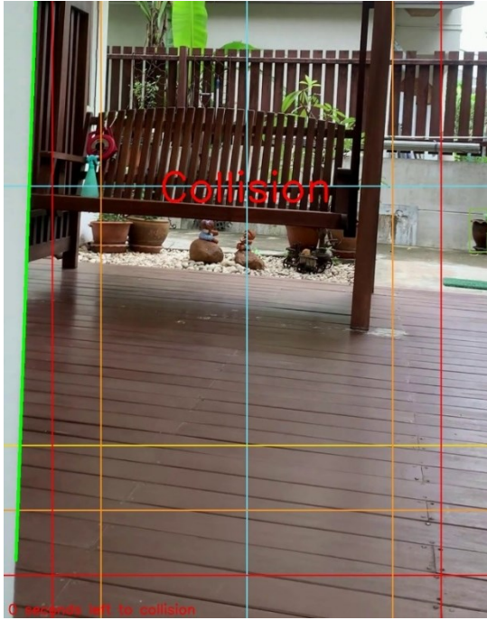
Figure 4. Obstacles that Canny can detect are outlined in the green line. In this figure, there appears an alert that means the edge of the pillar reaches the red left line.
