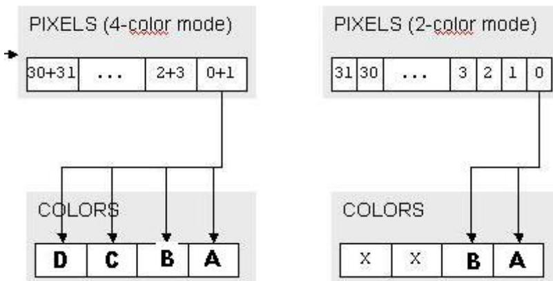
Now, exactly one of these bytes A, B, C, or D is output at some configurable 8 pin group (I/O 0..7, 8..15, 16..23) Be careful with group 24..31 the use of which is also possible.
