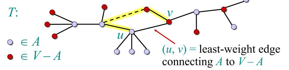
Consider the unique simple path from u to v in T. Swap (u, v) with the first edge on this path that connects a vertex in A to a vertex in V - A.
