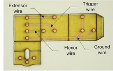
Fig. 14. Planar structure for the main body. Four electric wires are embedded: extensor, trigger, flexor, and ground wire.
