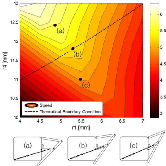
Fig. 12. Speed at takeoff with respect to various  $r_1$  and  $r_4$  values. In the region above the dashed line (e.g., point a), the latch of the robot cannot operate. On the dashed line (e.g., point b), the latch of the robot is unstable. The actual robot was fabricated at point c, considering the margin for a stable latch.
