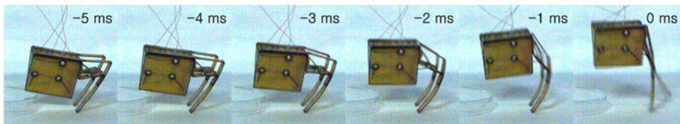
Fig. 17. Sequential pictures of the jumping motion (1-ms time intervals).
