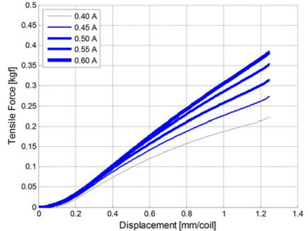
Fig. 5. Force–displacement curve for a single coil of the extensor spring with respect to various input currents. The stiffness increases proportionally to the amount of current input.
