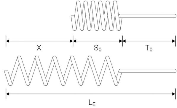
Fig. 8. Design of the extensor:  $L_E$  is the length of the extensor, which is the sum of the tendon length  $T_0$ , spring initial length  $S_0$ , and spring displacement  $X$ .
