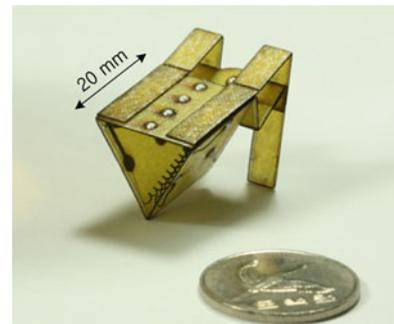
Fig. 1. Robotic prototype based on a flea-inspired catapult mechanism for miniature jumping robots. The diameter of the coin is 26.5 mm.
