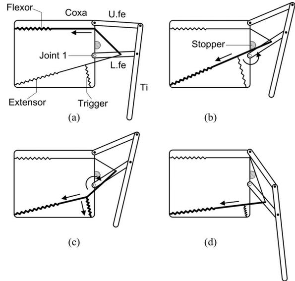
Fig. 3. Schematic design for miniature jumping robots based on a flea-inspired catapult mechanism. Three SMA springs function as artificial muscles: the extensor, trigger, and flexor. U.fe is the upper femur, and L.fe is the lower femur. Joint 1 was specially designed so that the extensor spring can pass through the rotational axis.
