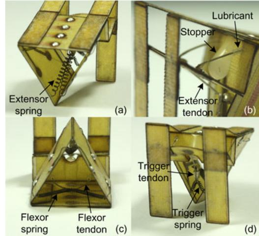
Fig. 15. Close views of the prototype. Each SMA spring is linked to each tendon and arranged in the body. Stopper and lubricant are attached to the body.
