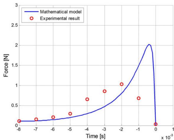
Fig. 19. Vertical reaction force profiles of the mathematical model and actual robot. The profile of the actual robot was shifted to set the time at takeoff to zero.
