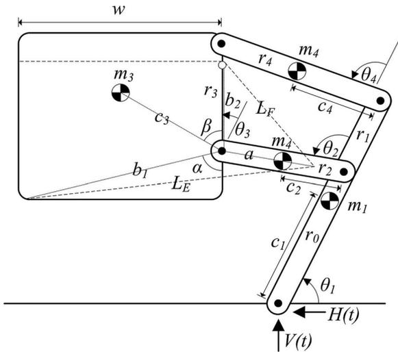
Fig. 7. Schematic of the robot. The robot uses a four-bar mechanism.  $L_E$  is the length of the extensor, and  $L_F$  is the length of the flexor.
