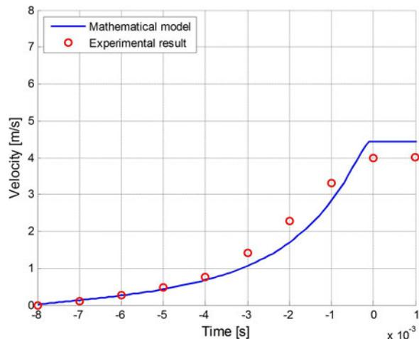
Fig. 18. Vertical velocity profile during takeoff. Both profiles of the mathematical model and actual robot were shifted to set the time at takeoff to zero.
