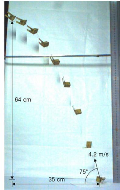
Fig. 16. Sequential pictures of the jumping motion (40-ms time intervals).
