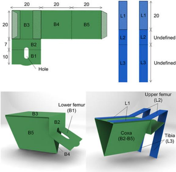
Fig. 6. Body design for miniature jumping robots based on a flea-inspired catapult mechanism. Planar structures become a 3-D structure when folded. Dashed regions are for adhesion.
