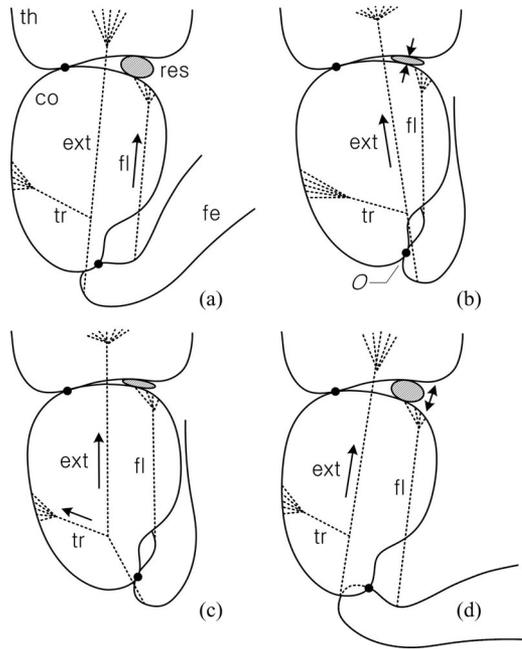
Fig. 2. Schematic of a flea's catapult. Three links are connected serially: th is the thorax, co is the coxa, and fe is the femur. A resilin pad (res) is located between the thorax and coxa, which function as a compression spring. Three muscles are arranged in the leg: fl is the flexor, ext is the extensor, and tr is the trigger muscle.
