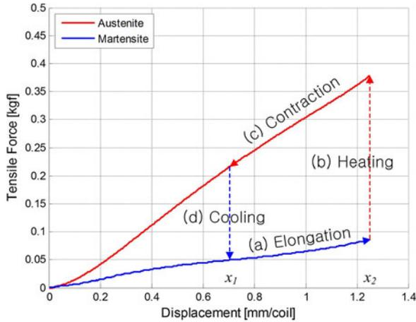
Fig. 4. Force–displacement cycle curve for a single coil of the extensor spring.
