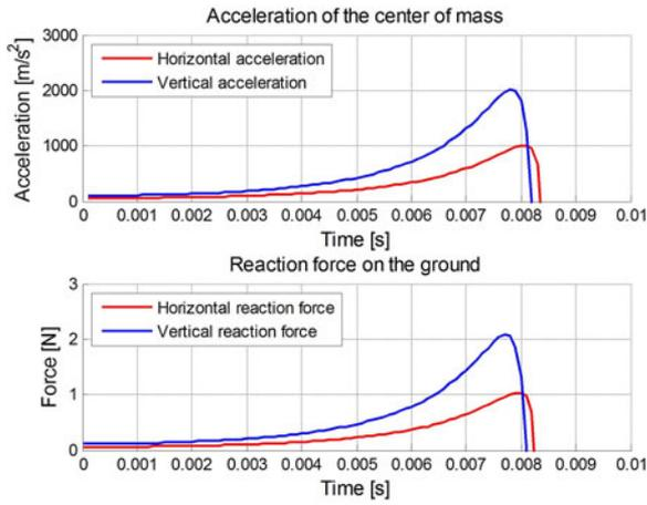
Fig. 10. Acceleration of the robot's center of mass and reaction force from the ground ( $r_1 = 5.5$  mm and  $r_4 = 11$  mm).
