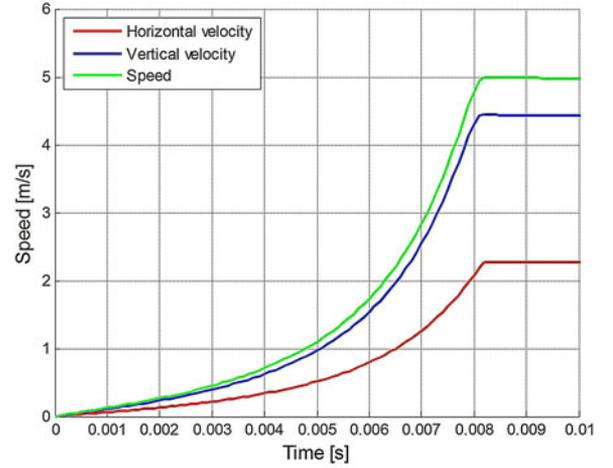
Fig. 11. Velocity of the robot's center of mass ( $r_1 = 5.5$  mm and  $r_4 = 11$  mm).
