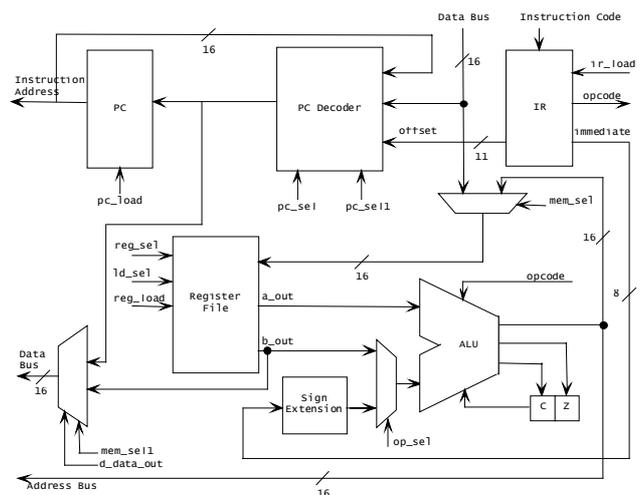
Figure 3 the architecture of S2 processor
