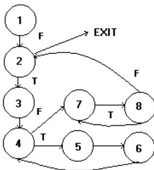
Figure 1 the data flow graph of the sieve program
