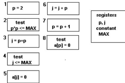
Figure 2 the computation node of the sieve program
