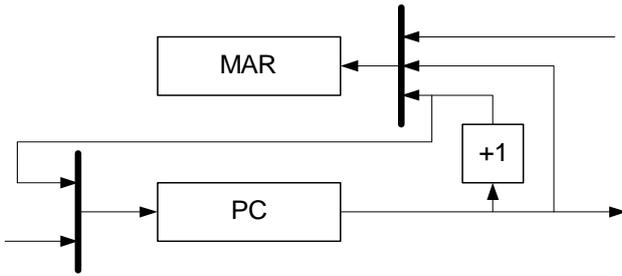
Fig. 3 show circuit changed by add adder at pc
