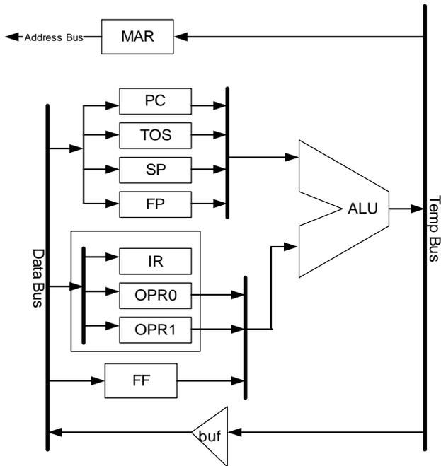
Fig 1 the micro architecture of the stack processor
