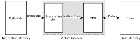
Fig. 1: Virtual machine with translation unit
