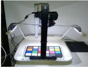
Fig. 1. The color measurement system calibration
