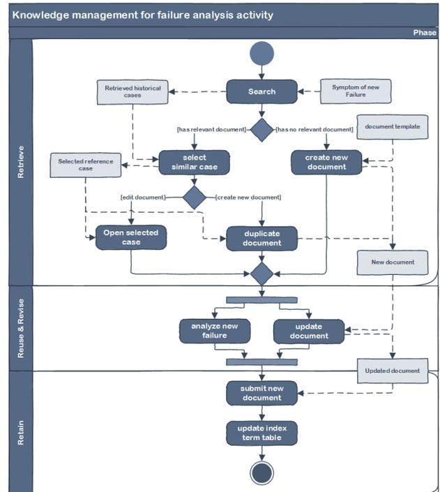
Fig. 6. Activity diagram to explain the user workflow.
