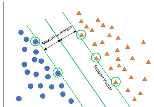
Fig. 1. Support Vector Machine that separate the hyperplane to classify the class with maximum margin
