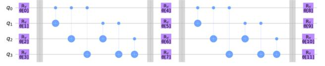
Fig. 2. RealAmplitudes circuit with two repeated circuits, Layer of RY-gates followed by CNOT-gates is applied on every pair of a qubit. The circuit has a total of 12 trainable parameters.
