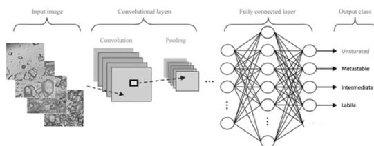
Fig. 2. CNN. of crystal prediction, output 4 classes.
