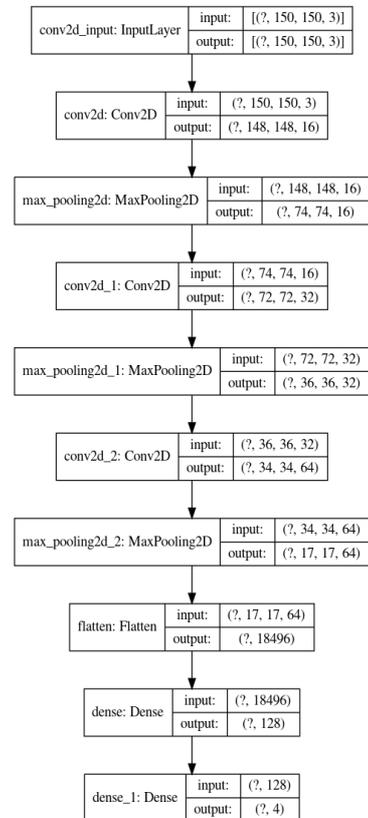
Fig. 6. Structure of model simple DCNNs.
