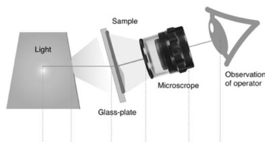
Fig. 3. Camera with x10 microscope.
