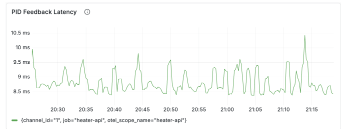
Fig. 8. Measured latency between Heater API and Thermometer API during a PID loop.
