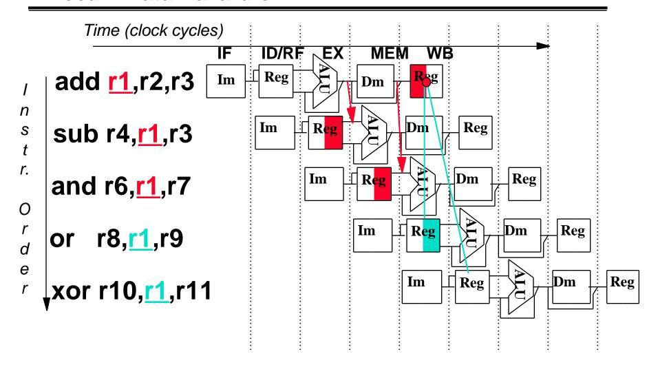
With MIPS R3000 pipeline, no need to forward from WB stage
