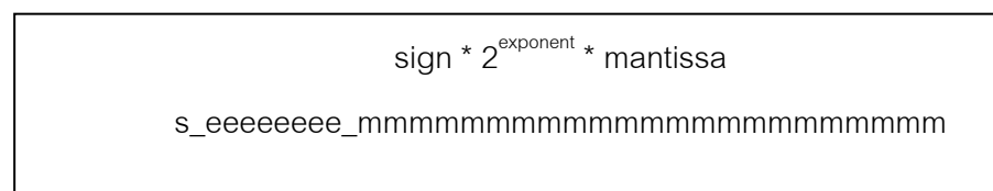
Figure 7 A 32-bit number of IEEE754 format for floating point calculation
