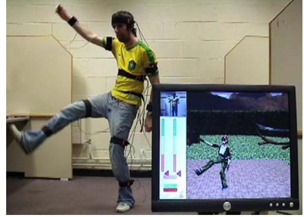
Figure 3 Real Time Motion Capture and Rendering
