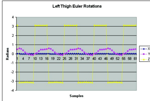
Figure 3. The yellow signal is an Eulerian version of a quaternion flipping around \pi .
